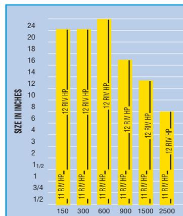
According to size and rating, port shape can be:
