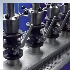
**Starline** is able to perform cryogenic testing in house or particular test under immersion according to API6A. Monitoring of tests is possible with cameras and recorded testing parameters.
