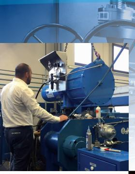
**Starline** testing area is equipped with multihead benches and separated control stations to test simultaneosly many valves or a single one especially for big sizes or to cover special testing procedures.
