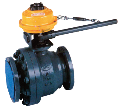
A temperature sensitive valve actuator with a self-contained energy source, for automatic valve operation in the event of a fire (fail-open positioning).
