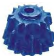
Type MG : Tooth type for medium to hard formations. Carbide inserts for gage protection.
