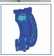
**Starline** uses the FEA for designing its Subsea valves. Finite Element Analysis (FEA) is a very important step of the development stage and ensures the best possible performance requirements. Valves operational problems, pressure/temperature related deformations and flow-related forces within a valve can be evaluated.
