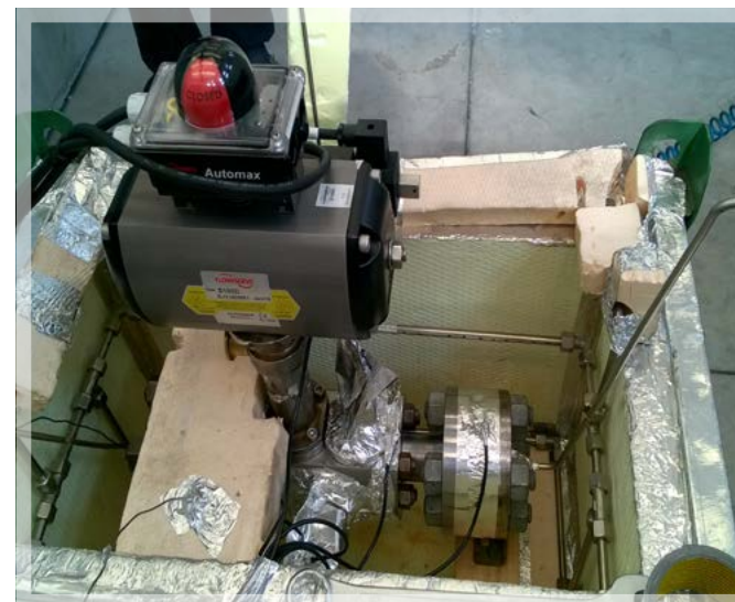
FET Prototype Test acc. to ISO 15158-1
