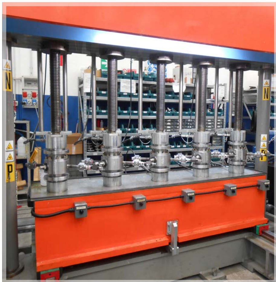
Multiple Stations Test Bench (Hydrostatic and Gas Test)
