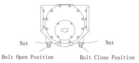
**Note:** Please note to tighten the bolt nut after adjusting the appropriate on/off position.
