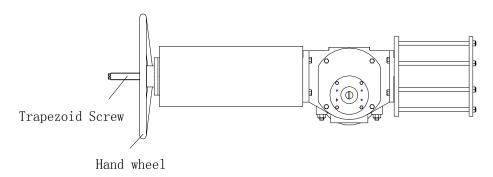
SY01F14 & SY01F16 after manual operation, screw out the trapezoid screw when it change to auto-operation way, to ensure the auto-operation smoothly realized. Avoid to screw out integral trapezoid screw, the valve open & close position will be influenced if the screwing is not in place.
