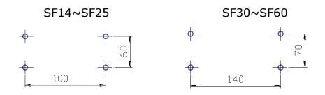
Top mounting pad of switchbox & E/P positioner
